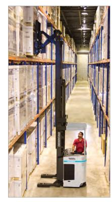
SRX offers advanced anti-rollback protection, ideal for minimizing push-back when placing loads. (See page 15 for details.)
