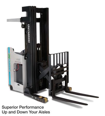
Specifically designed for the SRX, the AC motors are matched with a controller that's tuned to their precise torque and power curves. The result is quick acceleration, higher productivity, low energy consumption, and fast operating speeds.
