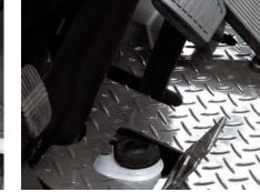
Two-piece diamond tread floorboard includes door to access brake fluid for visual level inspection and refills.
