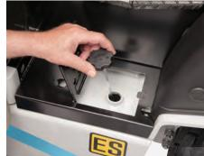
Access to hydraulic fluid located under door on right side step, for regular inspections and refills.
