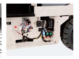
Side panel located behind left entry step offers access to relays and fuses.
